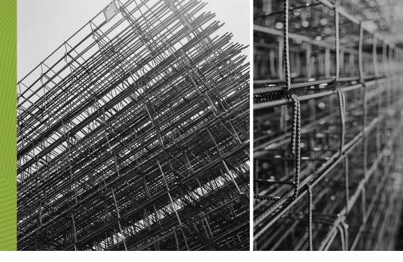
Is a reinforcement consisting of longitudinal and transverse wires welded together through resistance. Often it used as steel reinforcement in beams and columns.
