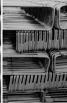
The stirrup are steel wire rods bent into a different shapes, which are placed perpendicular to the longitudinal reinforcement. They serve to position bars in the assembly of reinforcing elements. They are responsible to resist shear forces and diagonal tension that may affect an item.
