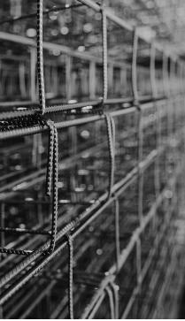
Is a reinforcement consisting of longitudinal and transverse wires welded together through resistance. Often it used as steel reinforcement in beams and columns.
